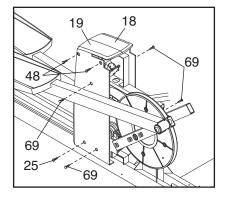
removed from; the Screws will later need to be reattached in the same holes. Carefully separate and remove the Flywheel Covers.
